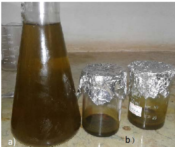
Fig. 2 Extraction of oil from filter cake by using dissolvent extraction method a) Leaching extraction
